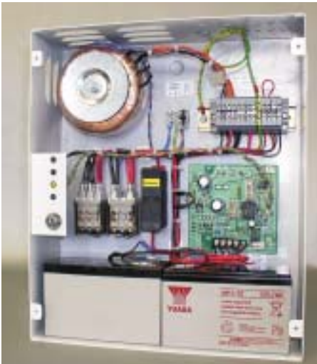
Group Control Panel
